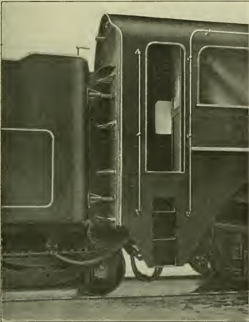
Vestibule Cab and Front End of Tender.
